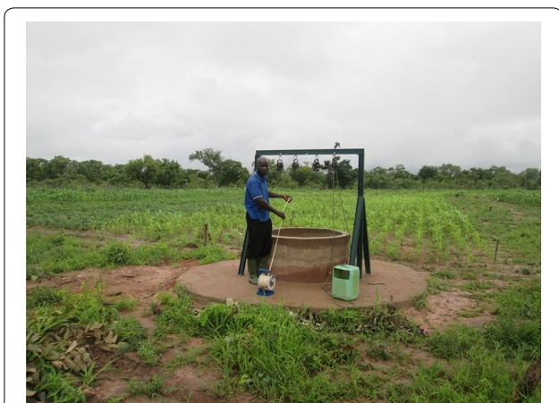
Fig. 5 Water level measurement using Dip meters in Flola Technology Park (TP) located in Bougouni district. Photo Credit Birhanu Zemadim, 2015. A TP is a research site developed by Africa RISING program in Bougounia and Koutiala districts to conduct experiments for research and demonstrate new technologies to the farming communities
